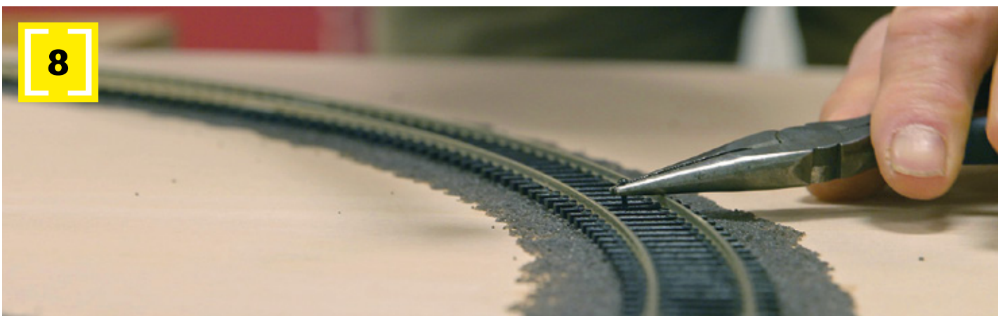
8 Gradually moving in an anticlockwise direction pin each piece of track down in turn. Having completed the oval you can now pin down the track in the siding. Remember not to knock the pin in too far. Allow the head of the pin to not quite touch the sleeper.
