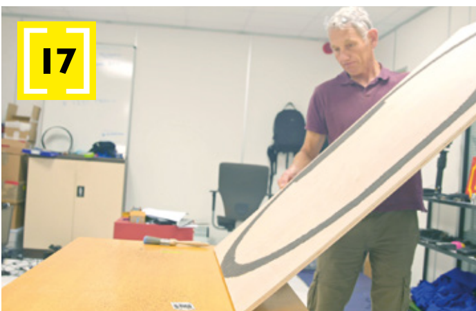
After applying the ballast to all of the track area wait for the glue to dry thoroughly and then tip the board up so that any loose ballast falls away. It is advisable to tip the board onto a piece of newspaper so that the excess ballast can be collected up for further use.
