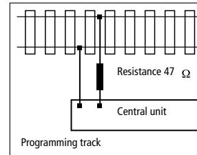
When programming using Lenz, Uhlenbrock or Arnold equipment, please refer to their programing instructions. If the error message "err02" is displayed during programming with Lenz or Arnold equipment, a 47 Ohmresistor (0.5) Watt or higher must be inserted between one of the two supply cables and the programming track.
