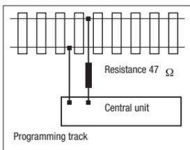
When programming using Lenz, Uhlenbrock or Arnold equipment, please refer to their programming instructions. If the error message "err02" is displayed during programming with Lenz or Arnold equipment, a 47 Ohmresistor (0.5 Watt or higher) must be inserted between one of the two supply cables and the programming track.
